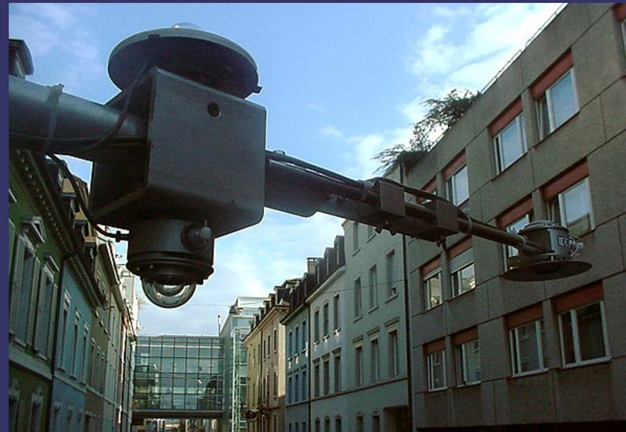
Full radiation components are measured once on top (33m) and also inside the canyon. Here, the sysem measuring directly over the street level at a height of 3.2m is shown. Photographed towards E. 6.12.01.
