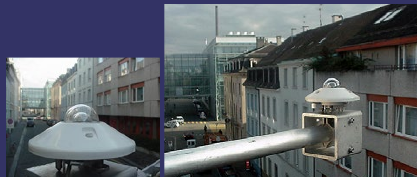
An additional Pyranometer (CM11) below rooftop at 12.4m (z/zH~0.8). Photographed towards E. 6.12.01.
