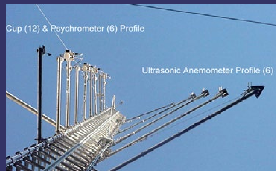
Upper part of the profile with 12 cup anemometers and 6 psychrometers. 6.12.01.
